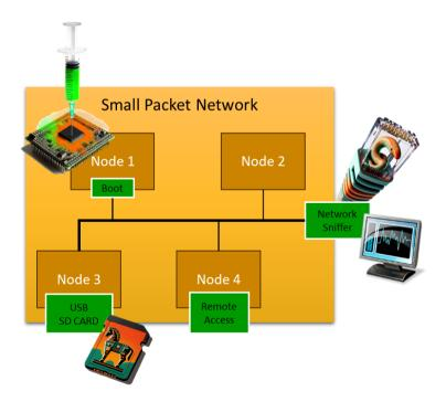
Anyone with physical access to the networking cable can easily install additional network interfaces that can "sniff" (read) all communication and inject or replay commands and other communication objects.
