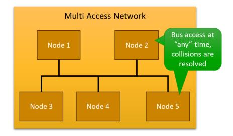
In CAN based systems, the arbitration process uses an address priority. The CAN frame with a higher priority wins the arbitration process.
