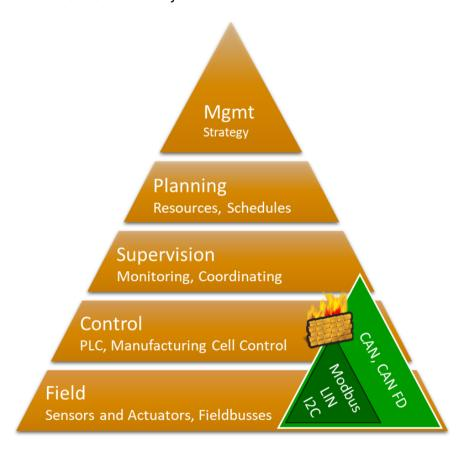
More generically the small-packet networks provide communication channels for microcontrollers to off-chip components. The serial or bus interfaces directly available on-chip with many microcontrollers include popular technologies such as I2C, SPI, LIN, Modbus, CAN and CAN FD.
