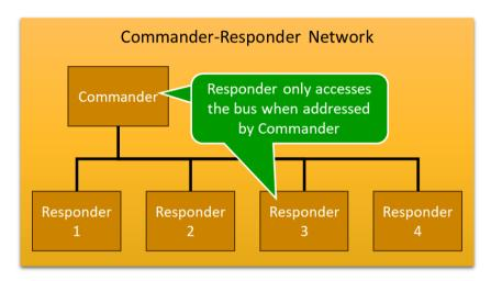
In SPI communication this is done by a chip select line, in I2C or Modbus an address value is used with which the commander can address a single Responder. Responders only communicate, if they received an appropriate command by the Commander. In these systems the Commander is fully responsible for the network access. Commaders decide when and why to address which of the Responders.
