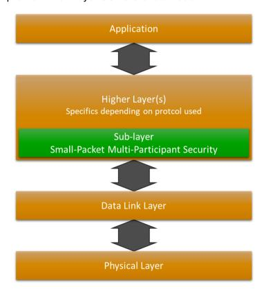
To achieve highest security levels and follow the security by design principle, additional security measures must be considered in the higher layer protocols. Here especially communication for configuration and network management require additional protection. Devices must be able to recognize the integrity of their own configuration.
