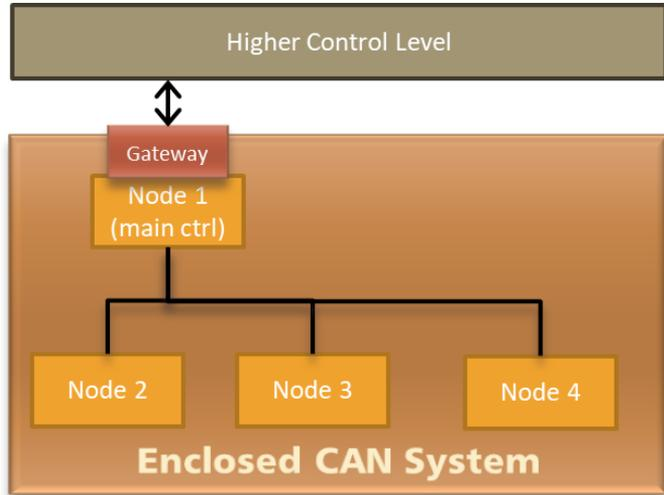
The communication consists of service, network management and process data communication. Process data communication is frequent and has real-time requirements. Service data communication is infrequent and typically happens during system startup or maintenance. Network management communication includes system startup commands, emergencies or alerts and heartbeats.
