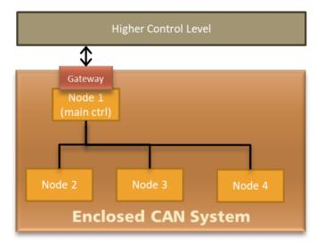
The communication consists of service, network management and process data communication. Process data communication is frequent and has real-time requirements. Service data communication is infrequent and typically happens during system startup or maintenance. Network management communication includes system startup commands, emergencies or alerts and heartbeats.
