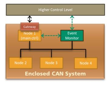
control unit using a separate serial communication channel. This communication is secured by a combination of TLS-PSK (Transport Layer Security based on pre-shared keys, RFC 4279) and cTLS (Compact TLS, RFC 9147). If supported by the hardware, the event monitor can also directly report to the higher control level using a state-of-the art secure communication channel.
