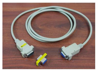
CAN\_H and GND need to be connected. Often RS232 cables like shown above can be used with gender changers. (NO Null-Modem cable!).
