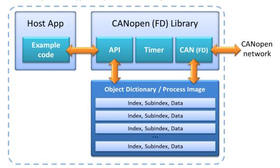
The figure above illustrates the operation blocks of the CANopen examples. The object dictionary and process image layout is configured using the CANopen Architect utility, which generates the .h configuration files needed by application example and library. The example application has access to the process image through the API of the CANopen library which also has direct access to it when transmitting or receiving data on the CANopen network side.
