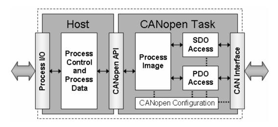
The Host implements the main process control application and directly handles all inputs and outputs to and from the application process. Using the CANopen API, the Host can exchange selected process data with the CANopen Task which is stored into the Process Image.
